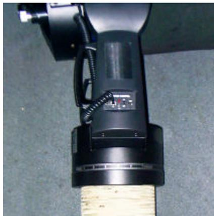
The plug mounts under the scopes base, just as if I was putting it on the tripod. The plug is then secured to the top of the pier with a threaded knob.
