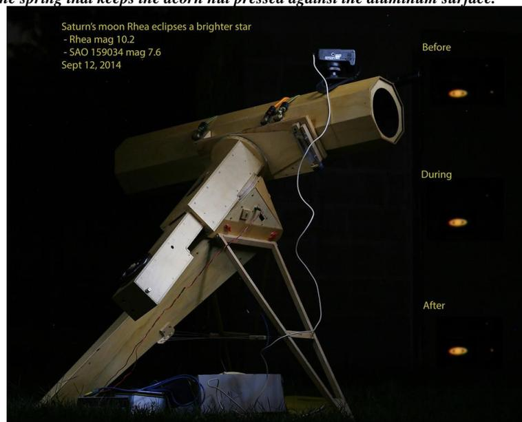
**Astrophotography in action: Capturing the occultation of star SAO 159034 / HIP 74007 (mag. 7.6) in the constellation of Libra by Saturn's moon Rhea (mag. 10.2). This image combines 1- and 5-second exposures during the event that lasted less than 19 seconds at 8:38pm EDT on September 12.**
