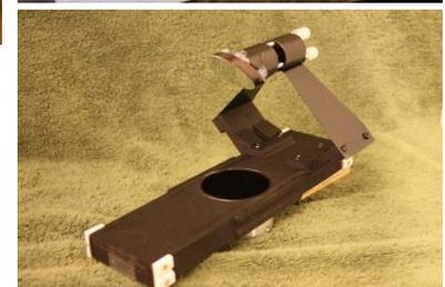
the collimation of the optical path. The slider would glide on a pair of brass rods and its lateral movement would be controlled by a threaded screw manipulated by the focuser wheel.
