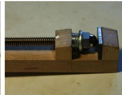
**(Left):** The Stellafane version had the acorn nut, but not the sheet of aluminum. **(Center and Right):** The post-Stellafane version shows the plastic bushing used to control the spring that keeps the acorn nut pressed against the aluminum surface.
