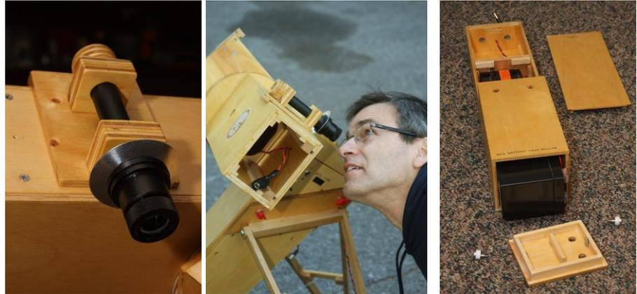
*The Polar Alignment scope (left) clips on to the Dec axis for use (center), and is then put away. The counterweight of the battery is then hooked up and inserted in the Dec axis box (seen above, empty). The counterweight assembly (right) stays in place by friction; there is no toe-saver! Thumb-screws secure the bottom and the battery is charged in place with the charger kept in the accessory box. Air vent holes are provided to vent any discharge gases.*
