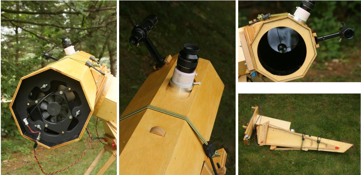
*The cooling fan for the mirror cell (left), the barrel focuser on the sled, whose lateral movement is controlled by the focuser wheel visible in the middle (center), the look down the OTA at the mirror (top right) and the compact folded disposition of the Mount (right), that being a prime objective. Beauty as seen through the optics, both celestial and terrestrial (below). Clockwise from the left: The Dumbbell nebula (M27), the eastern end of the Veil nebula and a daylily in the garden.*
